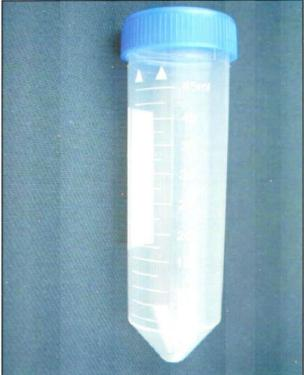
**Sputum container :** 50 ml Wide-mouthed, unbreakable, leak-proof, screw-capped made of translucent material
